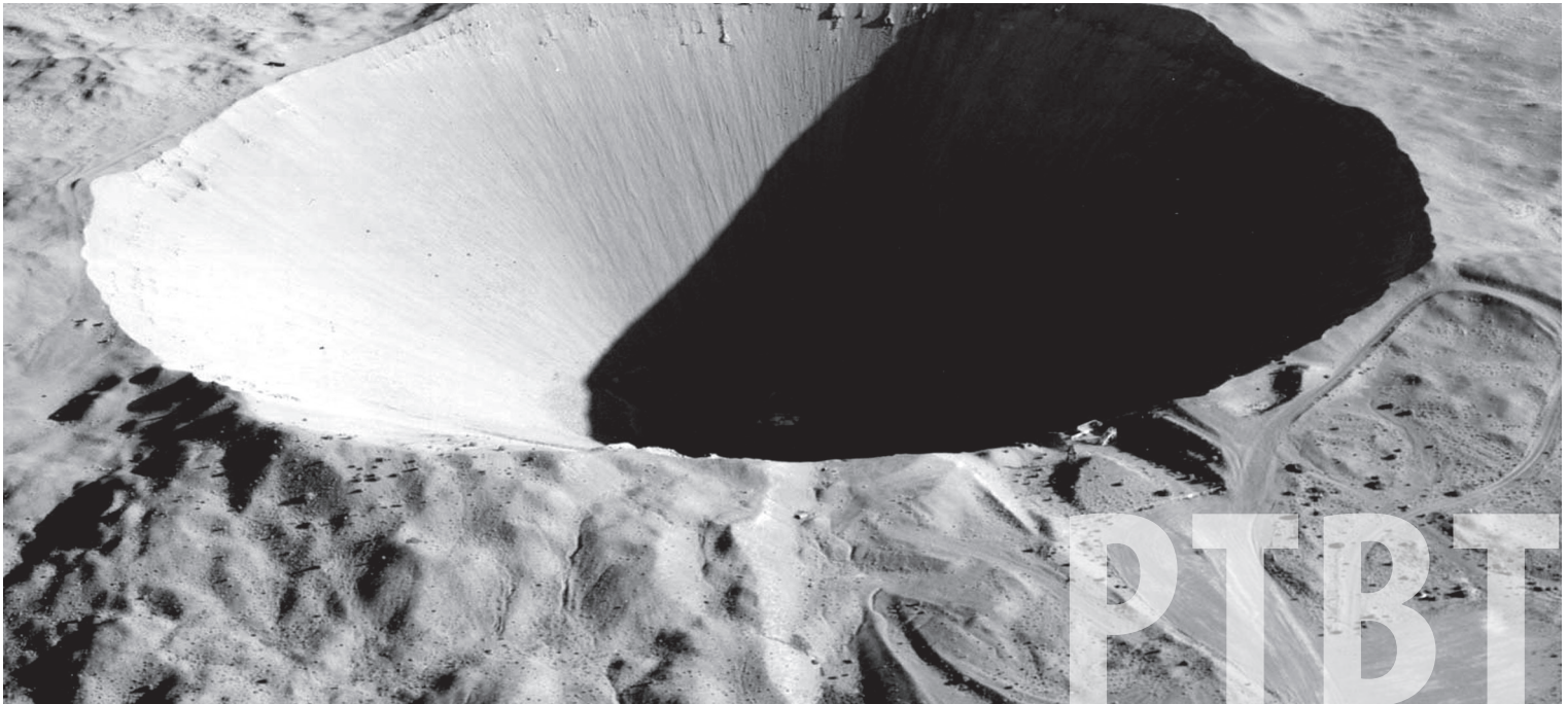
Crater from the 1962 "Sedan" nuclear test as part of Operation Plowshare. The 104 kiloton blast displaced 12 million tons of earth and created a crater 320 feet deep and 1,280 feet wide. United States Department of Energy
